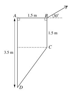
A uniform lamina of weight 15 N is in the form of a trapezium ABCD with dimensions as shown in the diagram. The lamina is freely hinged at A to a fixed point. One end of a light inextensible string is attached to the lamina at B. The lamina is in equilibrium with AB horizontal; the string is taut and in the same vertical plane as the lamina, and makes an angle of  $30^{\circ}$  upwards from the horizontal (see diagram). Find the tension in the string.
