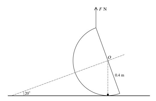
A smooth hemispherical shell, with centre O, weight 12 N and radius 0.4 m, rests on a horizontal plane. A particle of weight W N lies at rest on the inner surface of the hemisphere vertically below O. A force of magnitude F N acting vertically upwards is applied to the highest point of the hemisphere, which is in equilibrium with its axis of symmetry inclined at 20° to the horizontal (see diagram).
