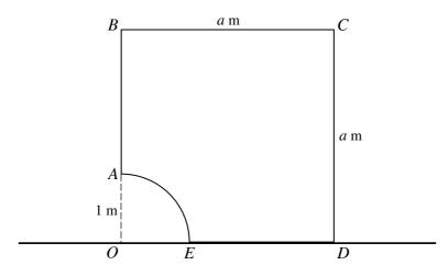
ABCDE is the cross-section through the centre of mass of a uniform prism resting in equilibrium with DE on a horizontal surface. The cross-section has the shape of a square OBCD with sides of length a m, from which a quadrant OAE of a circle of radius 1 m has been removed (see diagram).
