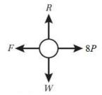
**b** The magnitude of the driving force is eight times the magnitude of the resistance force, so
