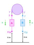
Let's build our equations for each object (object A and object B) before worrying about what the question is asking for. What they are asking for will come out if we build the equations correctly. We can ignore the purple tensions since they are acting on the pulley and we aren't needing to consider the pulley for this question (this is only when the questions talks about the forces exerted on the pulley).
