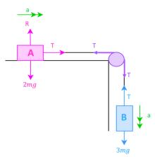
Let's build our equations for each object (object A and object B) before worrying about what the question is asking for. What they are asking for will come out if we build the equations correctly. We can ignore the purple tensions since they are acting on the pulley and we aren't needing to consider the pulley for this question (this is only when the questions talks about the forces exerted on the pulley).
