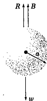
FIGURE 2.3.5 A body falling in a dense fluid.
